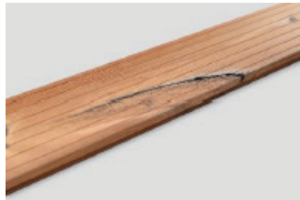
Large bark ringed knots are graded to B-quality.
