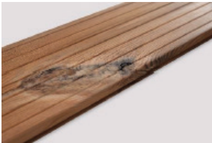
Boards with defects which clearly weaken the general quality appearance are sorted to B-quality.
